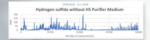
Hydrogen sulfide levels with use of HS Purifier Medium shows 1,14 % of the measurements is above 5 ppm against 41,6 % without use of HS Purifier Medium.
