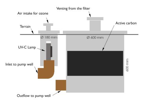
In the hydrogen sulfide filter under ground, the HS Purifier is placed so the UV-C produced ozone gets access to the pump well and is supplied to the well using the HS Purifier's ventilator.
