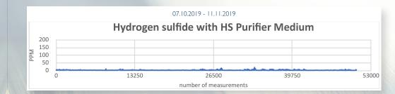
Hydrogen sulfide levels with use of HS Purifier Medium shows 0 % of the measurements is above 20 ppm against 16,4 % without use of HS Purifier Medium.
