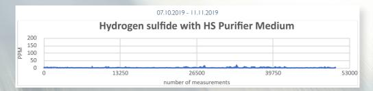
Hydrogen sulfide levels with use of HS Purifier Medium shows 0 % of the measurements is above 20 ppm against 16,4 % without use of HS Purifier Medium.
