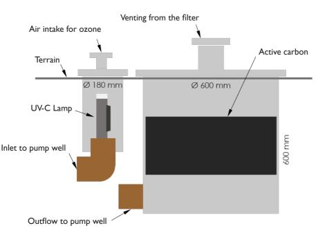
In the hydrogen sulfide filter under ground, the HS Purifier is placed so the UV-C produced ozone gets access to the pump well and is supplied to the well using the HS Purifier's ventilator.
